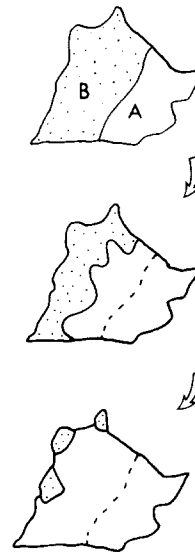
Fig. 7. Postulated mode of formation of 'left-over grains', after Urai (1983). A and B are quartz grains.
